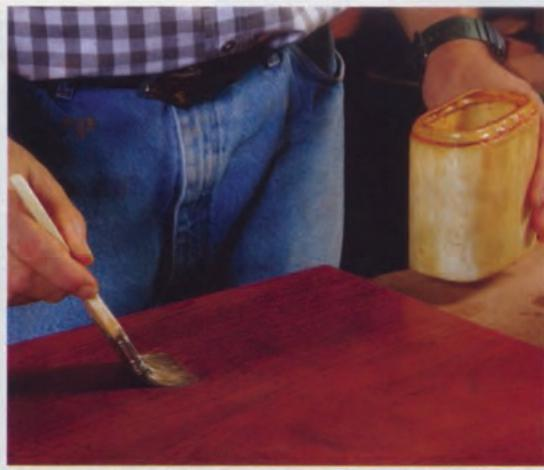
Brush on the oil. Don't be timid. The grain is going to really soak it up, so lay down a heavy coat (left). Then watch the surface for dull areas, where the oil has been completely absorbed. Add more oil to these areas until they are full (above). Finally, wipe off the excess when the oil begins to get tacky, about 45 to 60 minutes after you first applied it (below).
