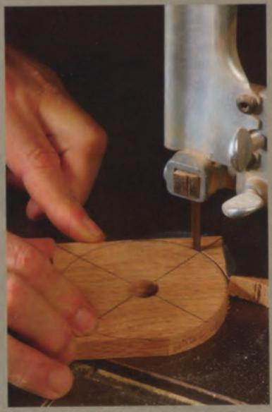
Cut it round. This lets you raise the blades higher above the table. The hole is for the arbor shaft (above). When re-stacking the blades and spacer, remember that the teeth on the blades must point inward (right).
