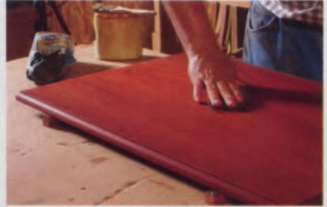
**Steel-wool rubdown.** It takes the place of wetsanding. Arceneaux uses 000 steel wool after the first two coats, and 0000 after the third.
