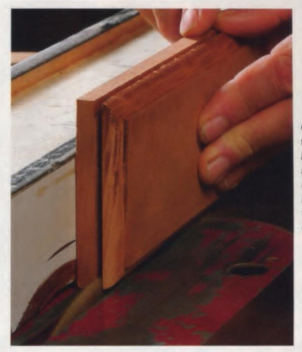
Cut a rabbet to create the lip. Make a second cut to complete the rabbet with the front flat on the table.
