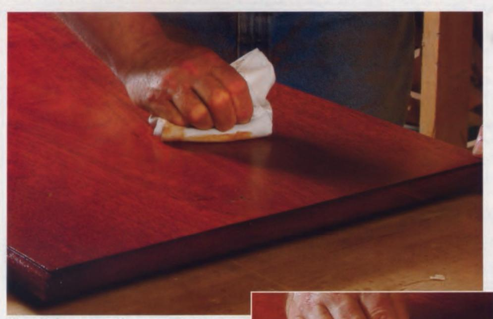
Wipe off the excess after every coat. Always use a clean rag, and do it when the oil is just getting a bit sticky (above). Use the steel wool between every coat (see opposite page) and finish with wax (right).
