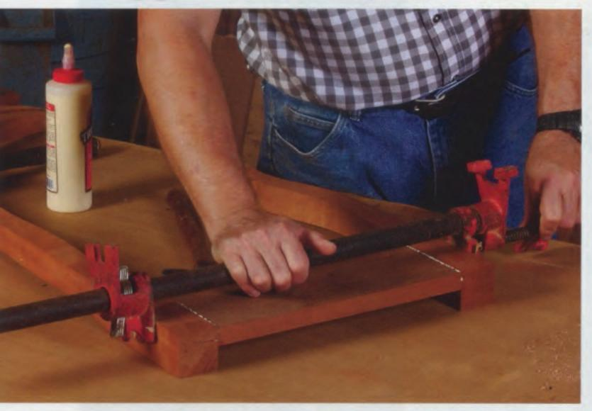
Two pegs hold the joint together just as well as a clamp while the glue dries, so ditch the clamps after the joints are pegged.
