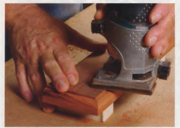
First profile the drawer front. Two scraps beneath the front create enough clearance to prevent the bit from contacting your bench.
