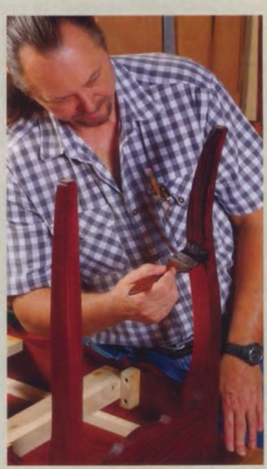
Brush on, buff off. A brush is faster than a rag and also does a better job getting into corners, edge profiles, and other details (above). A clean, soft rag is the right tool for buffing. Don't start until the wax has dried enough to haze over (below).
