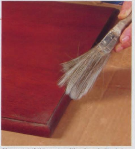
Clean out tight spots with a brush. The bristles of an unused brush knock steel-wool dust from corners, moldings, and routed profiles.
