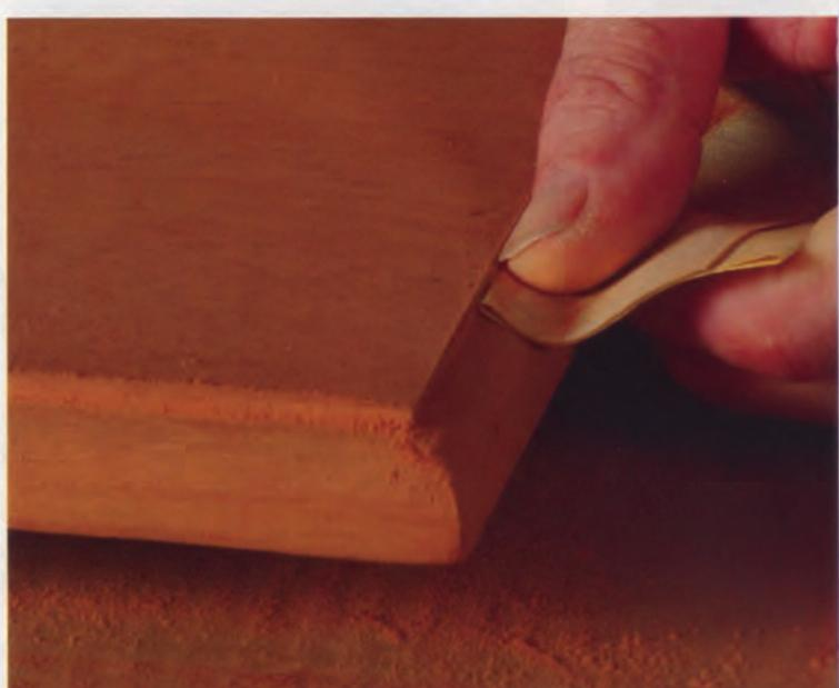
Save handsanding for the edges and details. A folded piece of sandpaper preserves crisp lines and gets into the tightest corner.
