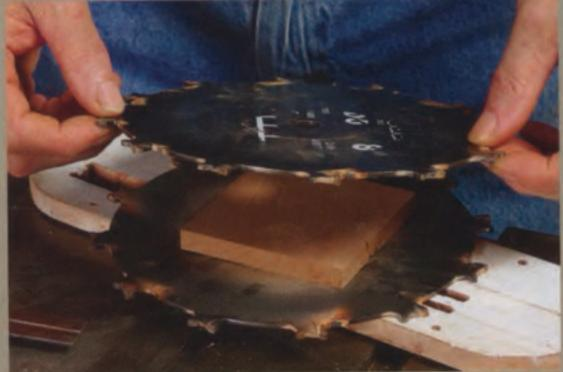
Mill a spacer so that its thickness matches the width of the mortising chisel. Place it between the two outside blades of a dado set (above), orienting the blades so that the high points of the teeth face inward. Assemble the sandwich and double-check the space between teeth (right).
