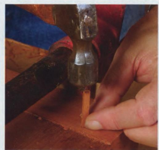
Sides first. Clamp a side stretcher between two legs (far left), pulling the joint tight and square. Then peg the joints right away (left). Arceneaux uses a square peg, but sharpens it in a pencil sharpener so that it is easier to start in the hole.
